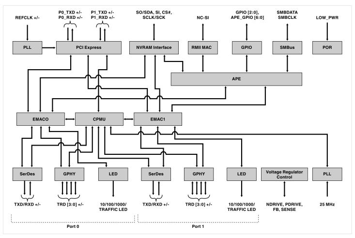
The BCM5718 is fabricated in a low-voltage 65 nm CMOS process, and integrates an efficient switching voltage regulator controller for core power supplies. Advanced power management features built into the BCM5718 enable minimizing the power consumption of the net-
