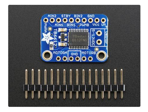
Comes as one assembled and tested breakout plus a small strip of header. You'll need to do some light soldering to attach the header onto the breakout PCB. Arduino, motors, and power supply not included.
