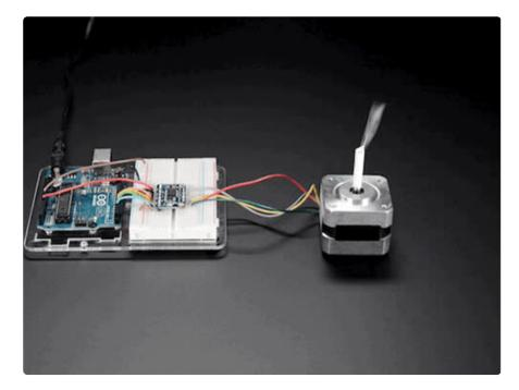
We solder on TB6612 onto a breakout board for you here, with a polarity protection FET on the motor voltage input and a pullup on the "standby" enable pin. Each
