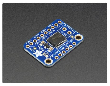
Fire four solenoids, spin two DC motors or step one bi-polar or uni-polar stepper with 1.2A per channel using the TB6612. These are perhaps better known as "the drivers in our assembled Adafruit Motorshield (http://adafru.it/1438) or Motor HAT (http://adafru.it/2348)" We really like these dual H-bridges, so if you want to control motors without a shield or HAT these are easy to include on any solderless breadboard or perma-proto.
