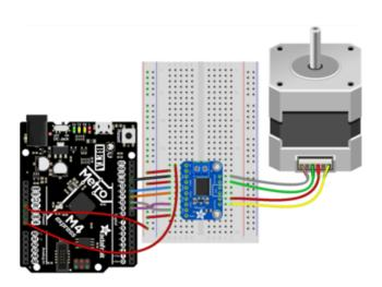
Board VM to Metro VIN Board VCC to breadboard power rail Board GND to Metro GND Board PWMB to breadboard power rail Board BIN2 to Metro D12 Board BIN1 to Metro D11 Board AIN1 to Metro D9 Board AIN2 to Metro D10 Board PWMA to breadboard power rail Breadboard power rail to Metro 5V Board MOTORA (two pins) to stepper coil (red and yellow stepper wires) Board MOTORB (two pins) to stepper coil (green and grey stepper wires) 9V power supply to barrel jack on Metro
