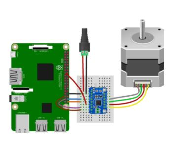
Board VM to positive terminal on barrel jack Board GND to negative terminal on barrel jack Barrel jack to 9V power supply Board GND to Pi GND Board SLP to Pi 3.3V Board AIN1 to Pi D19 Board AIN2 to Pi D26 Board BIN1 to Pi D20 Board BIN2 to Pi D21 Board AOUT (1 and 2) to stepper coil (red and yellow stepper wires) Board BOUT (1 and 2) to stepper coil (green and grey stepper wires)
