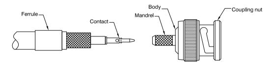
For insulated BNC's remember to put strain relief over the cable before crimping ferrule, then slide against body.
