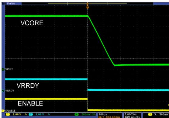
Figure 12: Enable-based Shutdown
