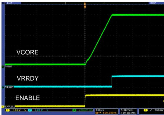
Figure 11: Enable-based Startup
